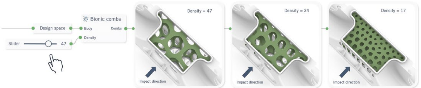
FIGURE 5 Bionic algorithm – construction algorithm applied to a design space and controlled through parameters (© ELISE)
